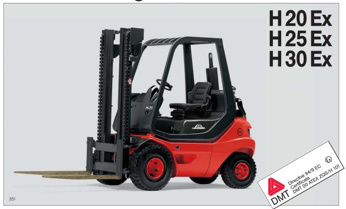
The Linde H20 Ex, H25 Ex and H30 Ex diesel forklift trucks designed for use in explosion-hazardous areas, are derived from the standard truck range H20, H25 and H30. These specialised versions therefore incorporate the same optimized performance and quality as the standard-production models: advanced engineering, exemplary ergonomics, long life, and economic operation.
